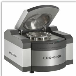
Provides non-destructive elemental analysis of particles, allowing us to determine their chemical composition and trace their origin—essential for root-cause investigations and corrective actions.
