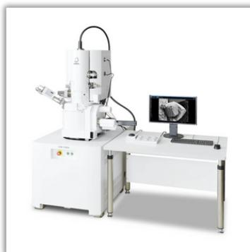
Delivers ultra-high-resolution imaging and morphology analysis at micro and nano scales. With EDS, SEM offers forensic-level insights into contaminant structure and composition.
